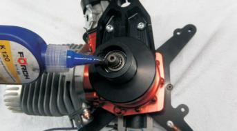
STEP 15 install the clutch bell
