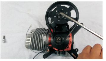
STEP 3 block the drive shaft behind the clutch bell with fitting pliers and open the nut with a fitting socket and wrench
