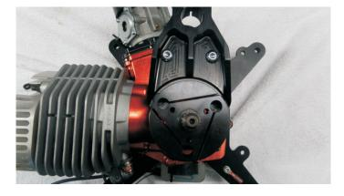
STEP 12 use a torque wrench and tighten the 2x bigger Torx screws with 22NM
