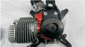
STEP 5 remove drive wheel and belt
