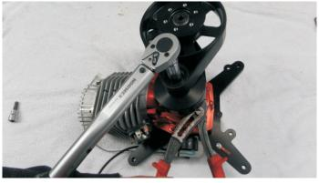
STEP 17 install the drive wheel with belt
