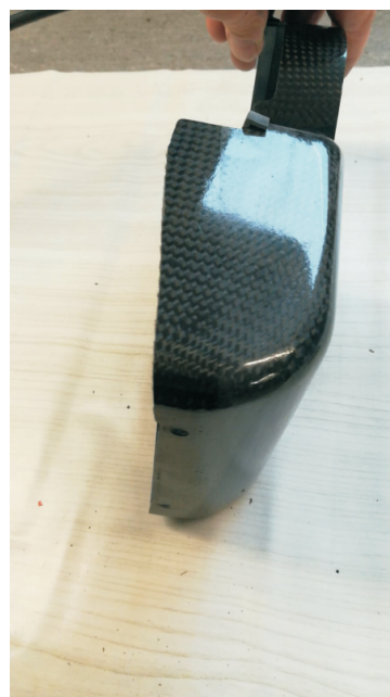
part after cutting and removing tape
