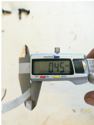
reference band to adjust gap with width of 0,45mm
