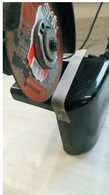
turn part to prepare for cutting on the other side
