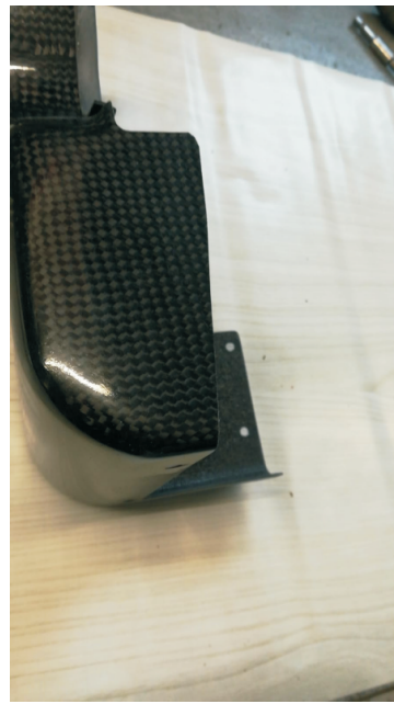
part after cutting and removing tape
