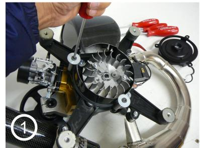
Well place starter and put bolts in position. Important! - use Loctite 243 thread locker to secure the bolts.
