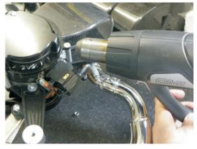
In general, only use quality tools (metric) to open/close the bolts. These bolts are glued with Loctite 243 thread locker, therefore hard to open. Open slowly and with care!
