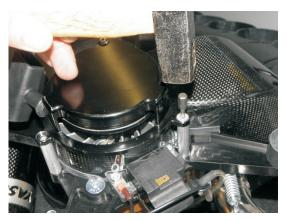
... take a Torx Bit size 20 and hammer it in into the damaged Inbus head. Well take care that it will go in as deep as possible.
