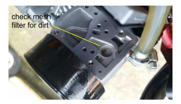
**Caution!** - A polluted mesh filter may cause the engine to start running to lean step by step with danger of overheating and melting the piston! We therefore recommend to check the filter at least every 10 hours of engine operation.
