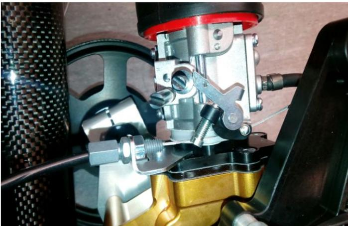
**Important note!** - connect fuel line with appropriate inner diameter 6mm (see picture), put tube over nipple only, no extra additional fitting needed. Check for a proper air-tight fit.
