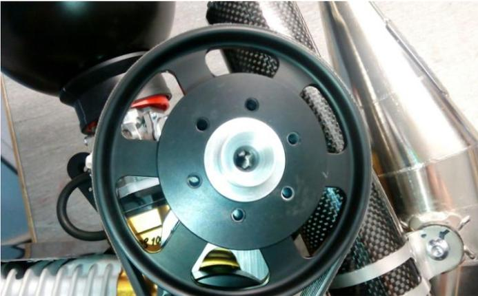
**Important note!** - use the proper bolts (not coming with the engine) with proper lengths (metric M6, Inbus type with washer, min. 8.8 quality) where the thread of the bolt goes min. 15mm and max. 25mm into the thread of the drive wheel.
