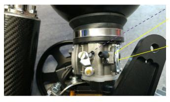
idle adjuster screw H jet adjuster screw (sealed with shrink tube or laquer)
